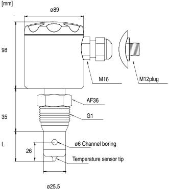
Insert length L = 40: Standard sensor shaft Insert length L = 87: Extended sensor shaft **LCDisplay** 999.9 mS/cm 139.9 °C Max. indication
