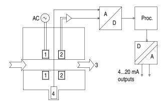
Inductive conductivity measurement is based on the principle of a transformer. The primary side of the transformer is controlled by an AC voltage generator.
