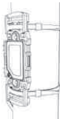
With cable ties
