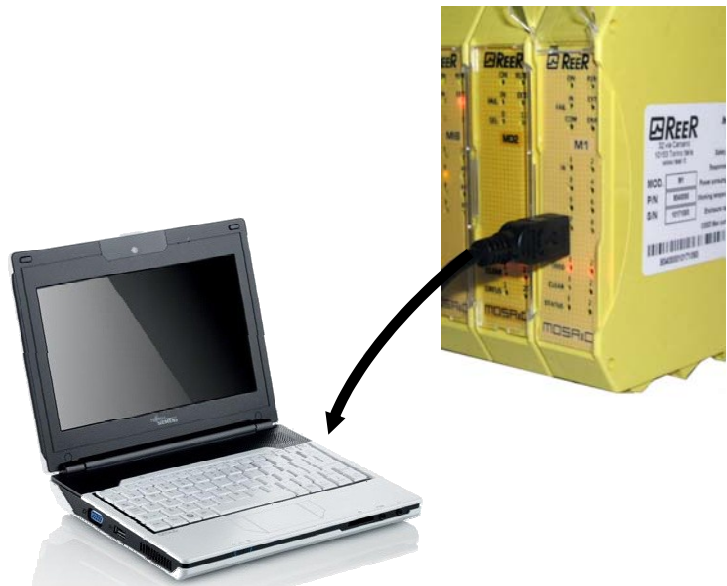
Figure 2 - USB 2.0 front panel connector
