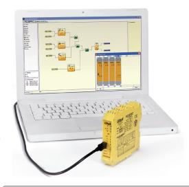
The Mosaic M1 master is equipped with a USB 2.0 serial bus for the connection to a PC on which the MSD (Mosaic Safety Designer) configuration software is held.
