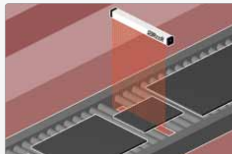
Measuring width and position of panels or slabs on roller/conveyor belt-borne material.
