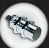
Capacitive sensors are suitable for the detection of metallic and non-metallic objects of all types. Even highly transparent glasses or liquids are easy to detect with a capacitive sensor. Only the dielectric conductivity of the target material is relevant: the greater the dielectric constant of a material, the higher the possible switching distances or the more reliable the detection.
