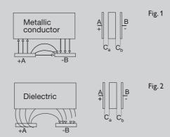
Capacitive sensors are actuated by both conductive and nonconductive objects. Objects made of conductive materials form a counter-electrode to the sensor's active face. This forms two capacities,  $C_{\Lambda}$  and  $C_{D}$  connected in series, with the electrode surfaces A and B (Fig. 1). The capacity of this serial connection is always greater than the capacity of the uncovered electrodes A and B.
